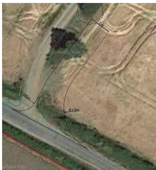
Figure 46: Junction Work Area: Sunnica East Site B on Elms Road for Staff Car Park
