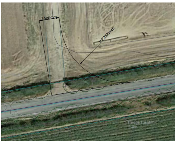
Figure 42: Junction Work Area: Sunnica East Site A on Beck Road
